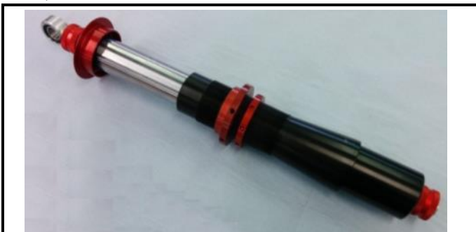
G6-1) Shock absorber dismounted
