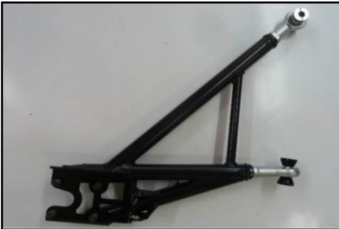
G5-1) Complete wishbone/arm front – dismounted
