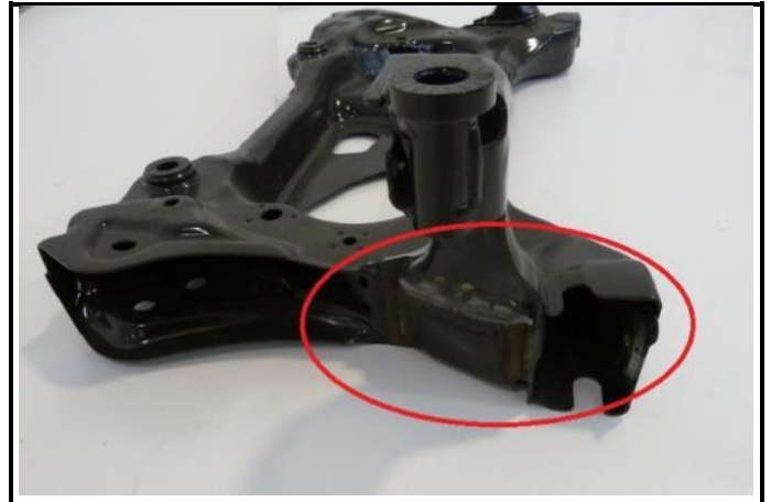
G2-6) Subframe – Supports' Modification
