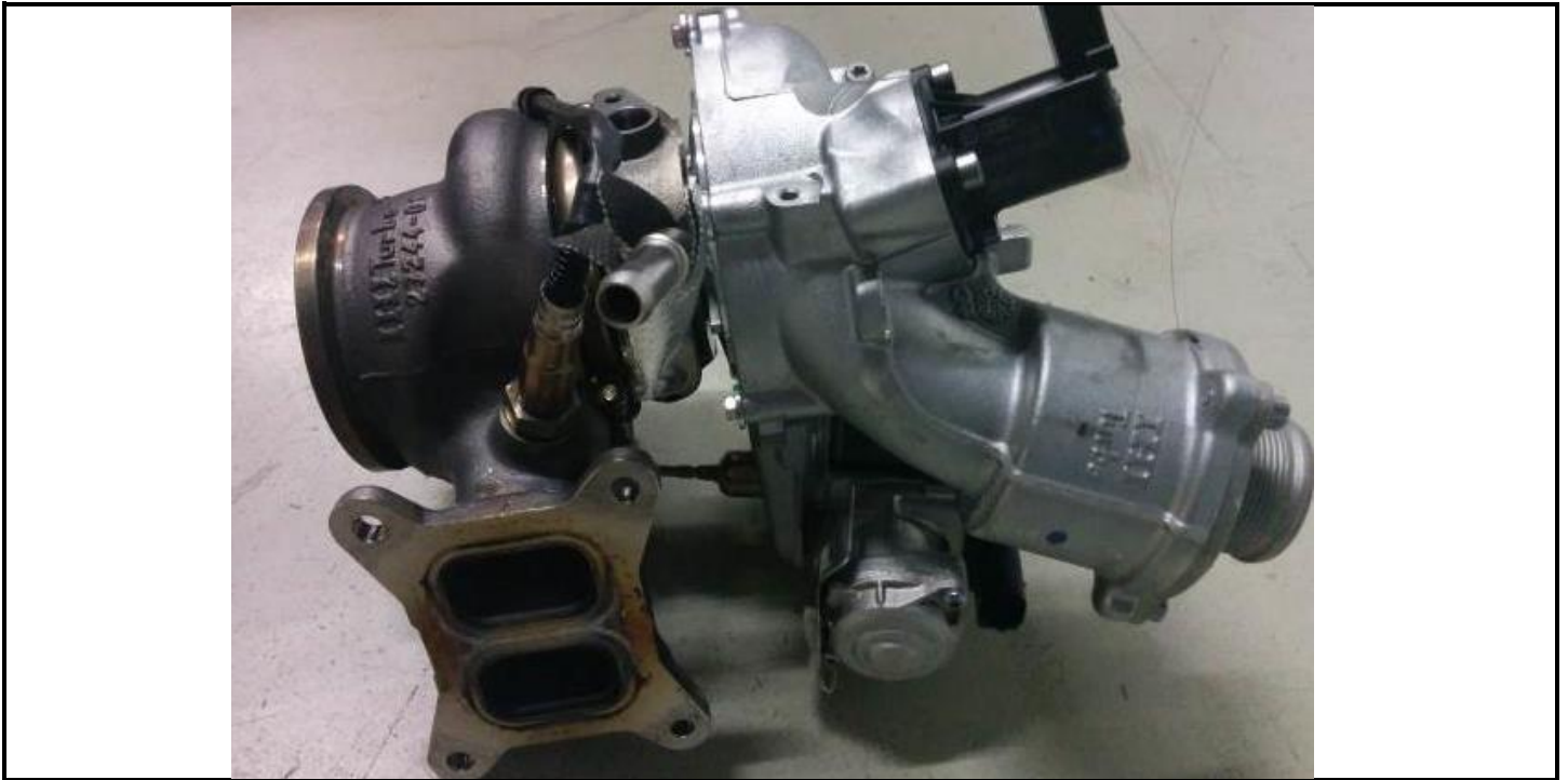
C15-3) Side view of complete turbocharger unit
