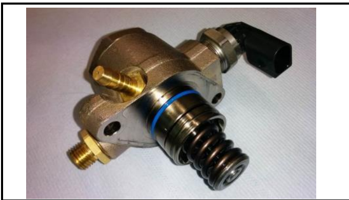
D2-1) Fuel pump(s) - dismounted
