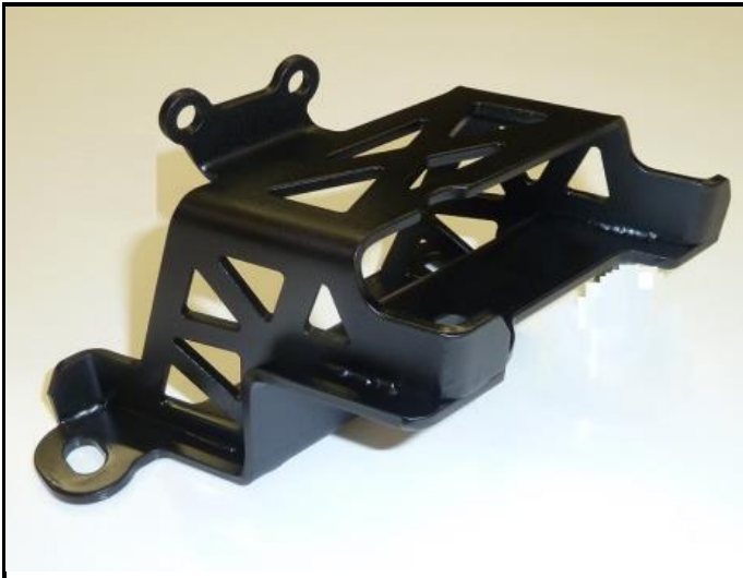
C2-3) Engine support 3 dismounted (photo)
