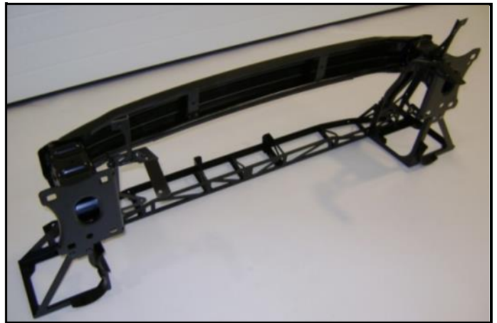
M15-6) Rear bumper brackets - rear view
