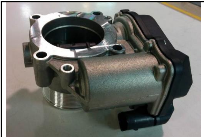
C11-3) Throttle unit - dismounted
