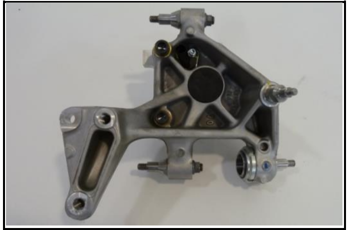
H3-4) Wheel bearing mounted
