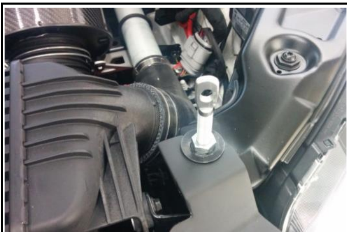
M5-1) Engine bonnet open - retaining support(s)
