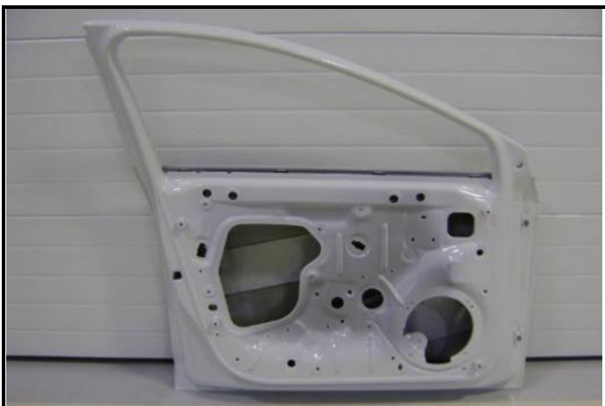
M7-1) Bare front door – inner face
