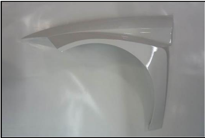
M6-1) Rear fender - dismantled
