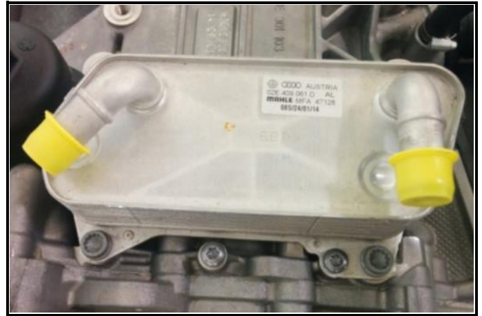
F2-8) Gearbox cooling – in location
