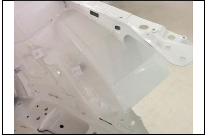
N4-3) Front suspension turret – top mount
