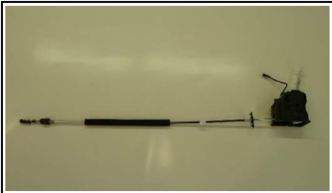
F2-3) Gearbox command - dismounted
