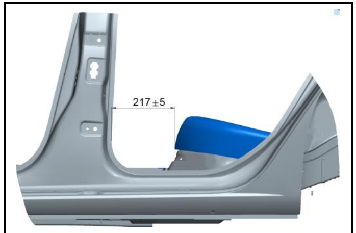
XII-A2) Longitudinal position of the original back seat
