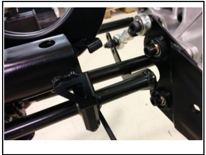
VIII-E2) Positions of the pivot points on the wishbone/arm
