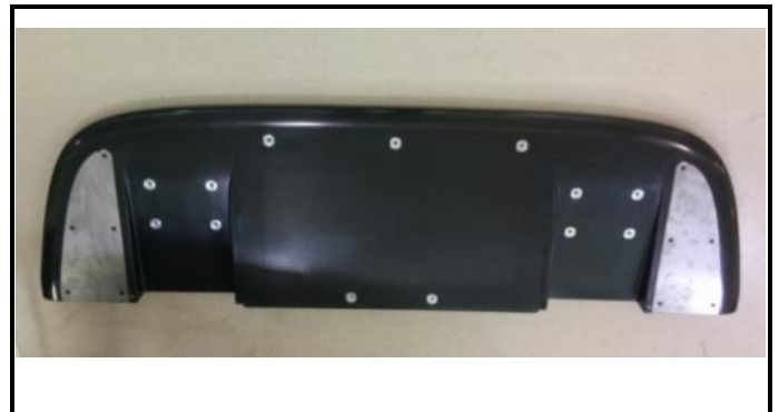
M15-2) Complete front splitter - dismounted
