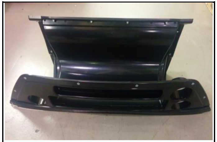
C13-6) Water cooler air ducts - dismounted
