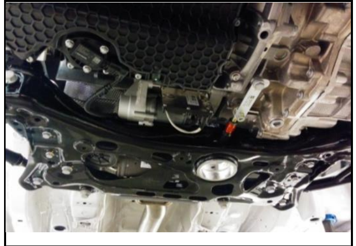
G2-4) Subframe – Modification of axle mounting points
