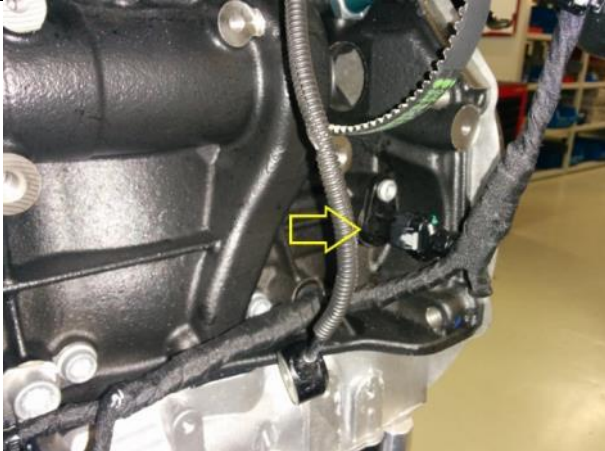
ENGINE SPEED SENSOR IN ITS LOCATION
