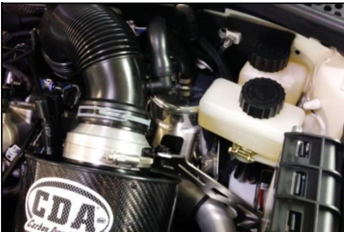
J8-1) Brake fluid tank(s) in location
