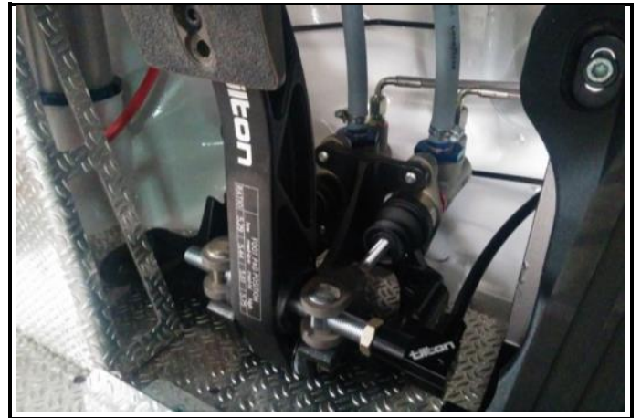
J5-2) Braking Regulator in location
