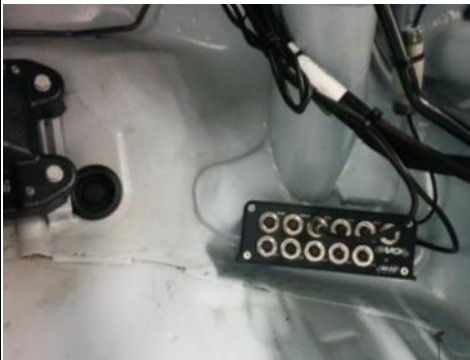
DATA LOGGING UNIT IN ITS LOCATION
