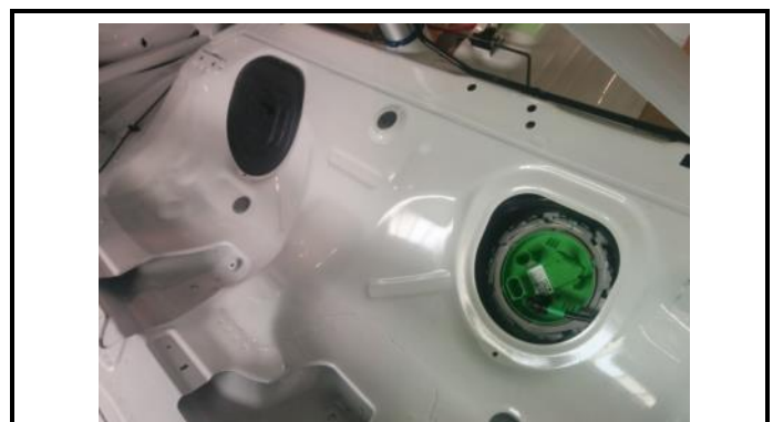
D2-4) Low pressure fuel pump(s) - in its location
