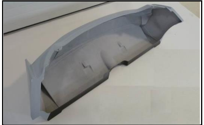
M11-2) Rear bumper - dismounted inner side
