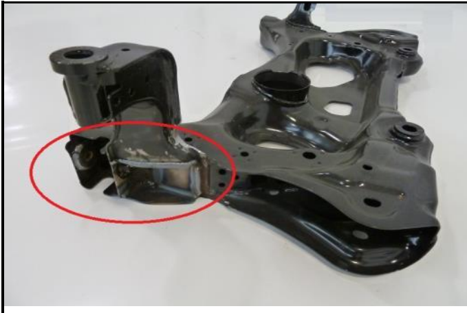
G2-5) Subframe – Modification of axle mounting points
