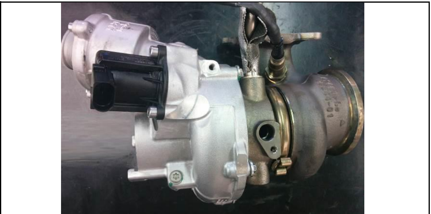
C15-1) Plan view of complete turbocharger unit
