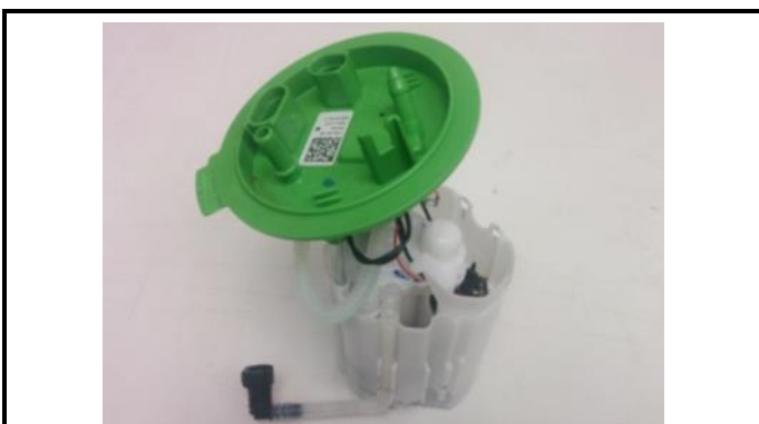
D2-3) Low pressure fuel pump(s) - dismounted
