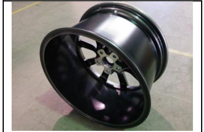
I1-4) Rear wheel attachment dismounted
