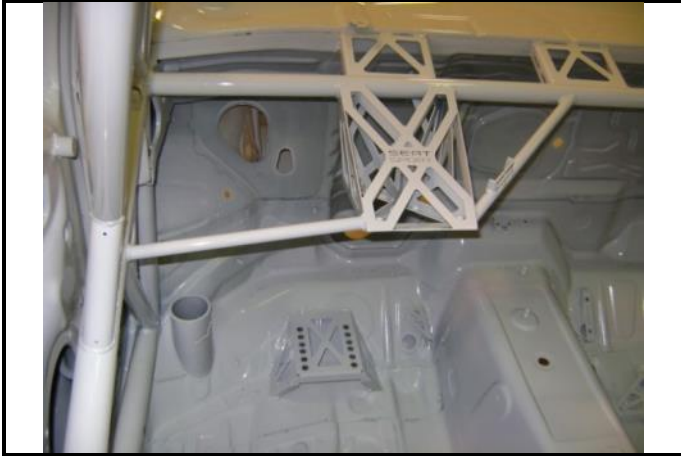
N4-2) Front member – Gearbox support
