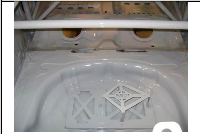
N1-9) Body shell identification plate
