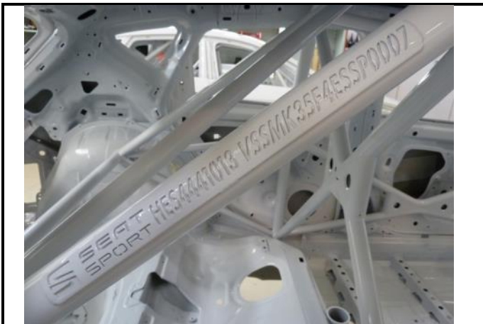
N1-9) Body shell identification plate
