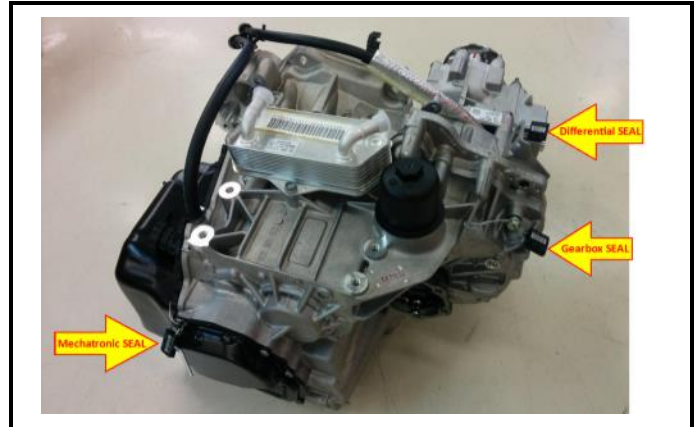
F2-4) Gearbox command - mounted
