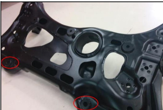
G2-5) Subframe – Modification of axle mounting points
