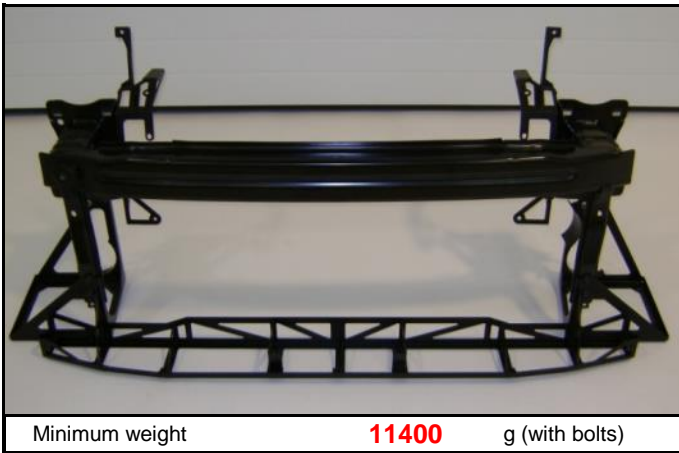
M15-5) Rear bumper brackets - front view
