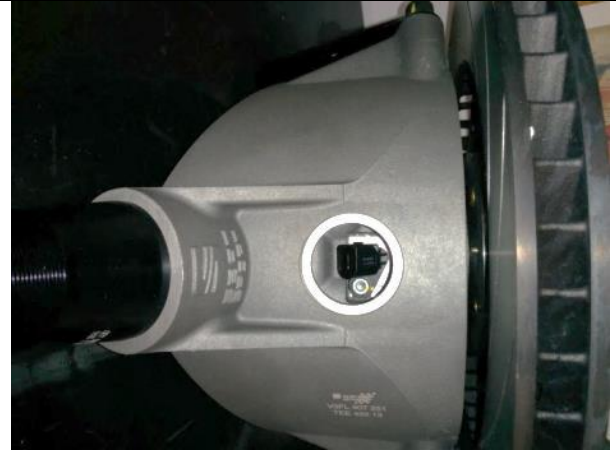
FRONT WHEEL SPEED SENSOR IN ITS LOCATION
