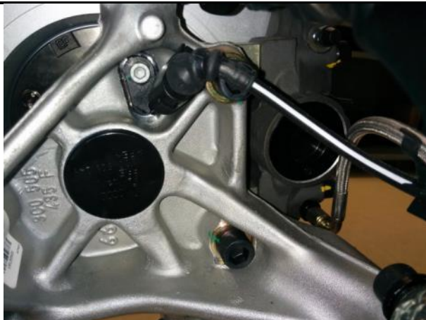
REAR WHEEL SPEED SENSOR IN ITS LOCATION
