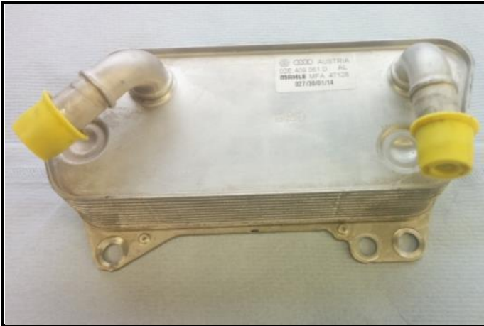
F2-7) Gearbox cooling – dismounted
