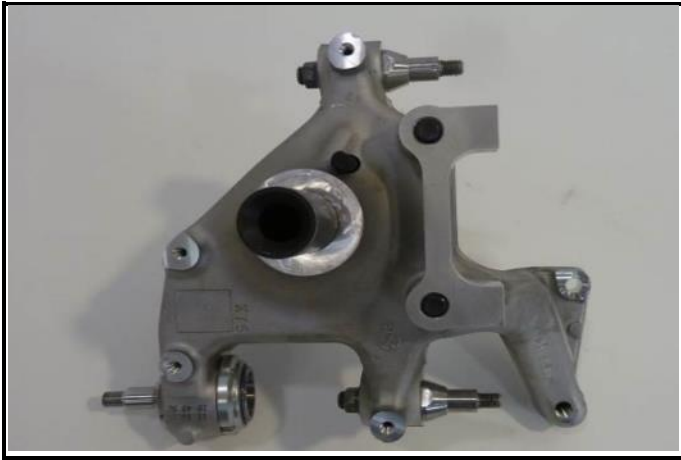
H3-3) Wheel bearing dismounted
