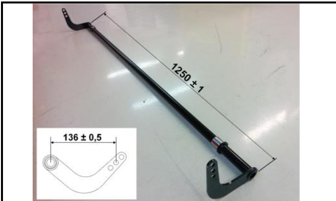
H7-1) Anti roll bar dismounted
