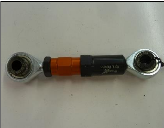
C2-3) Engine support 3 dismounted (photo)
