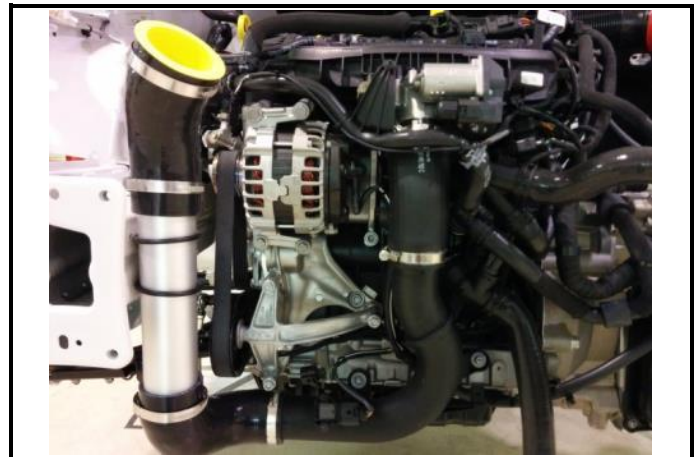
C11-9) Intake manifold & Air ducts - in location
