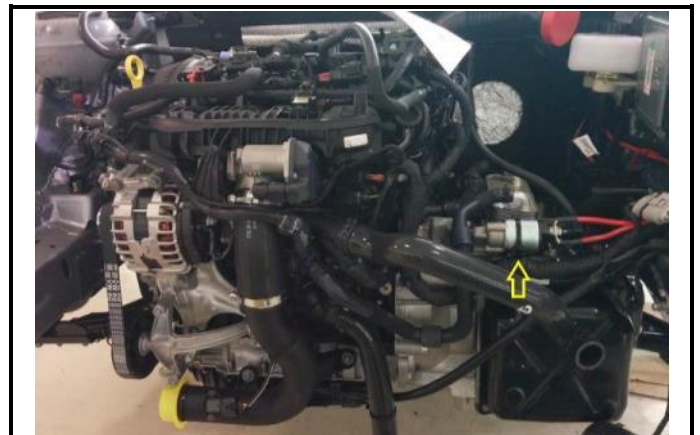
E1-4) Starter – mounted in its location
