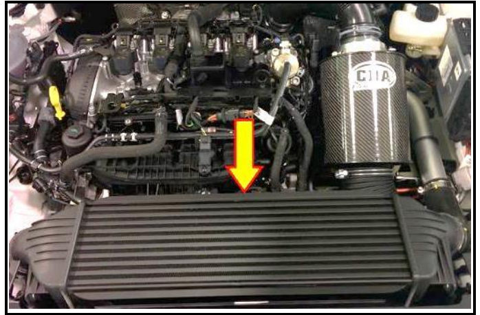
C15-10) Intercooler - mounted in its location with air ducts
