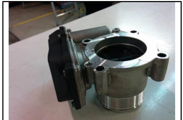
C11-4) Throttle unit - dismounted
